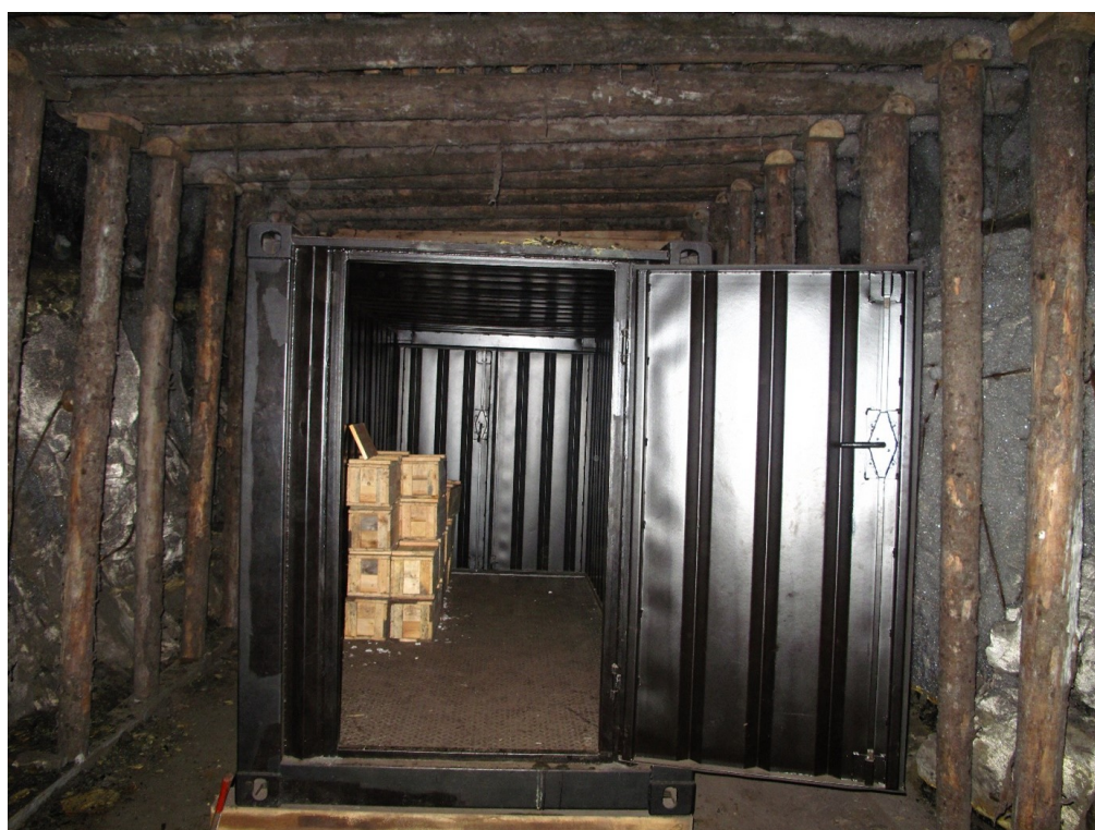
Figure 2. The history of conserving seeds in permafrost started in 1984, when backup samples of the Nordic Gene Bank seed collection were deposited in a steel container placed in an abandoned shaft of Cole Mine #3. The container is still in the mine, hosting some experimental seed samples while the backup collection has been moved to the Seed Vault. (Photo: NordGen)
